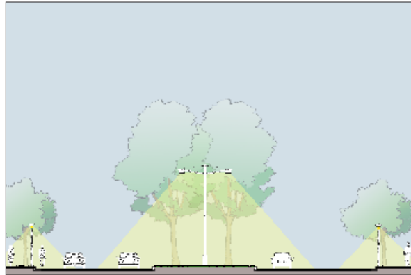
Auto-oriented street lighting (2Avii-3)
